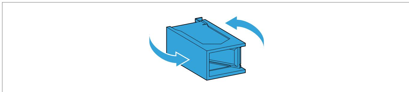
4. Take the old supply air filter (1) out of the filter module and dispose of it. Alternatively, remove the filter bracket, including the old supply air filter (2), from the filter module.
