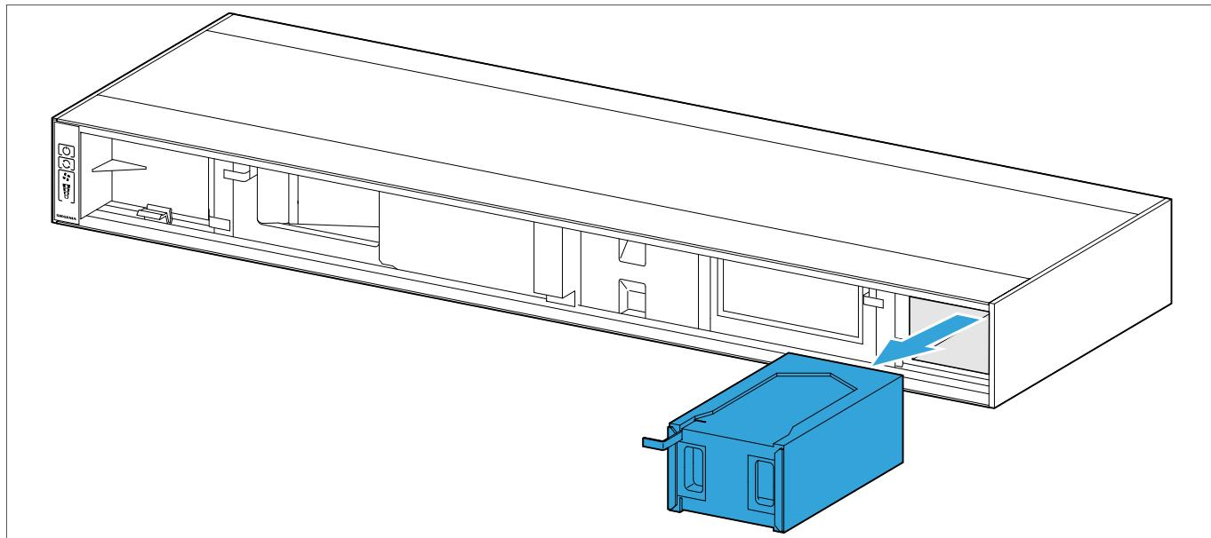
3. Rotate the filter module through 180°.
