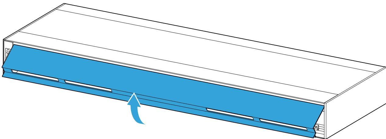
2. Take the filter bracket, including the old exhaust air filter, out of the device.
