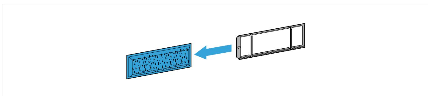
4. Insert the new exhaust air filter into the filter bracket.
