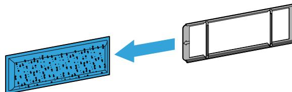
6. Insert the new supply air filter into the filter bracket.
