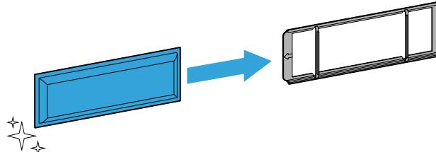
7. Insert the new supply air filter (1) into the filter module. Alternatively, insert the filter bracket, including the new supply air filter (2), into the filter module.
