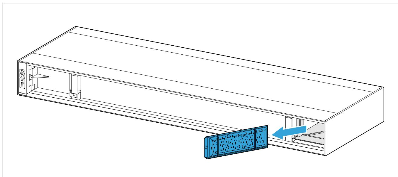
3. Take the old exhaust air filter out of the filter bracket and dispose of it.
