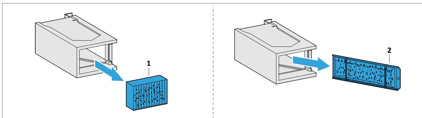
5. Take the old supply air filter out of the filter bracket and dispose of it.
